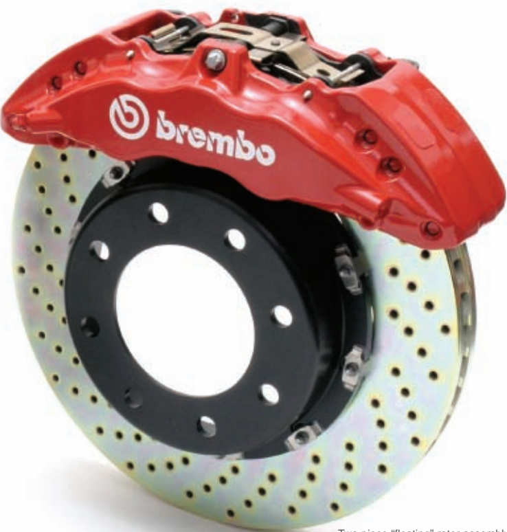
Two piece "floating" rotor assembly
